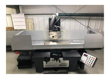
PTD employs Okamoto's latest in state-of-the-art precision surface grinders. Servo controlled Z axis allows for precise grinding with exceptional surface finishes. The 2 axis Fanuc controller allows us to grind shoulder and steps accurately. The GX and EXB models are a double V contruction rather than the standard flat and V .
