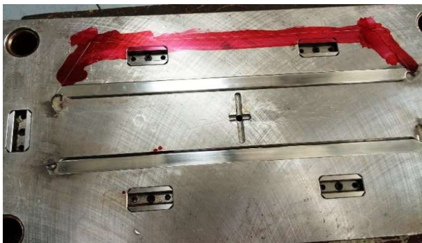
Revision to injection mold to make part 2" wider. Weld, machine and polish.
