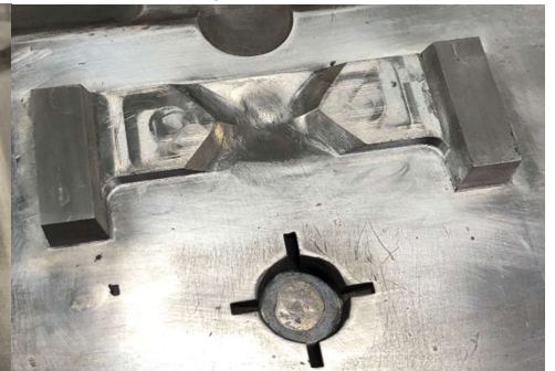
Revision to injection mold to make part 2" wider. Weld, machine and polish.
