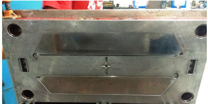
Revision to injection mold to make part 2" wider. Weld, machine and polish.
