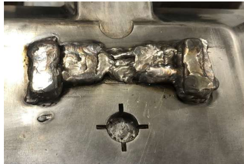
Revision to injection mold to make part 2" wider. Weld, machine and polish.
